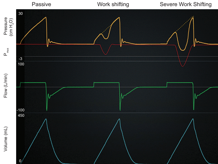
Fig. 8. Work shifting in volume control (VC) square flow waveform. Mode: VC-CMV. P_{mus} : graphic representation of patient-generated pressure. Passive breath: no P_{mus} . Work shifting: The pressure waveform is deformed toward baseline due to the presence of P_{mus} . It does not cross the baseline. Interrupted line demonstrates where the pressure waveform would be if P_{mus} was passive. The ventilator is still doing some amount of work on patient. It may be clinically appropriate. Severe work shifting: The pressure waveform is deformed due to the presence of P_{mus} ; the pressure crosses the baseline (PEEP). Under this circumstance, the patient is doing work against the ventilator. This is never clinically appropriate; it needs immediate clinician attention. Note: red P_{mus} line was overlaid by hand onto a ventilator screen image, and P_{mus} is shown inverted for clarity. CMV = continuous mandatory ventilation.
